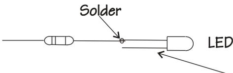
Short Leg is the Cathode. Cathode is connected to the Negative side of the Supply
