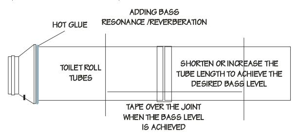
Generally, good quality sound reproduction on is more of an 'Art than a Science' as there are so many variables which can make phenomenal differences to the output quality, and again what works really well for a 'Fog-Horn' Module may be useless for a Heavy Ordinance Cannon. However with very simple and inexpensive experimentation the module will out-perform most of its competitors in both Sound Output Quality and expensive power consumption in the field.
