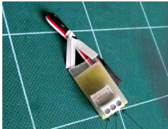
Normally Open Contact Common Contact Normally Closed Contact
